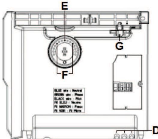
To prevent unauthorized changes to the settings, you can lock or limit the travel of control knob **C** and lock the slider **B**. To do this, remove the appliance from the wall bracket. On the back of the thermostat housing, pull out the pins **D**:
