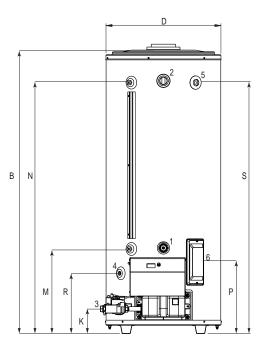
\*Optional flue pipe adaptors are available for DR-LL 90 to increase flue connection to 250mm (round draught diverter and box type 1 draught diverter)
