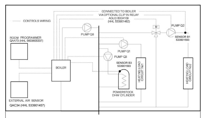
Figure E 1.3.3 - Schematic for Single Boiler (External 0~10V), Multi Circuit System
