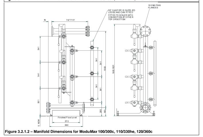
3.2.2 The Hamworthy Heating Ltd water manifold kit is designed to provide a compact solution for connecting the boilers to the gas supply and flow and return water connections. There are two kits specific to individual models. (Refer to the Installer's Guide 500005119 for specific details on the manifold kit. suitable for 150c/160he/200c/220/250c models)
