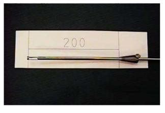
3. Ensure that an insertion distance of 200mm is set on the combustion analyser probe.
