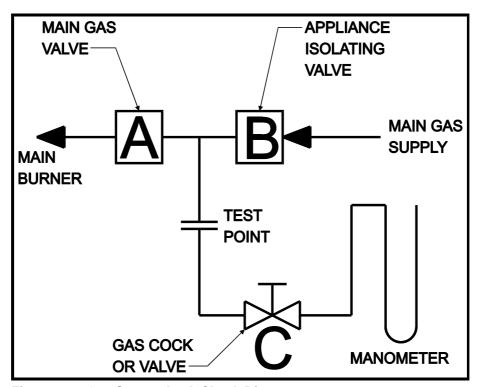
Figure 7.1 - Gas System Leak Check Diagram
