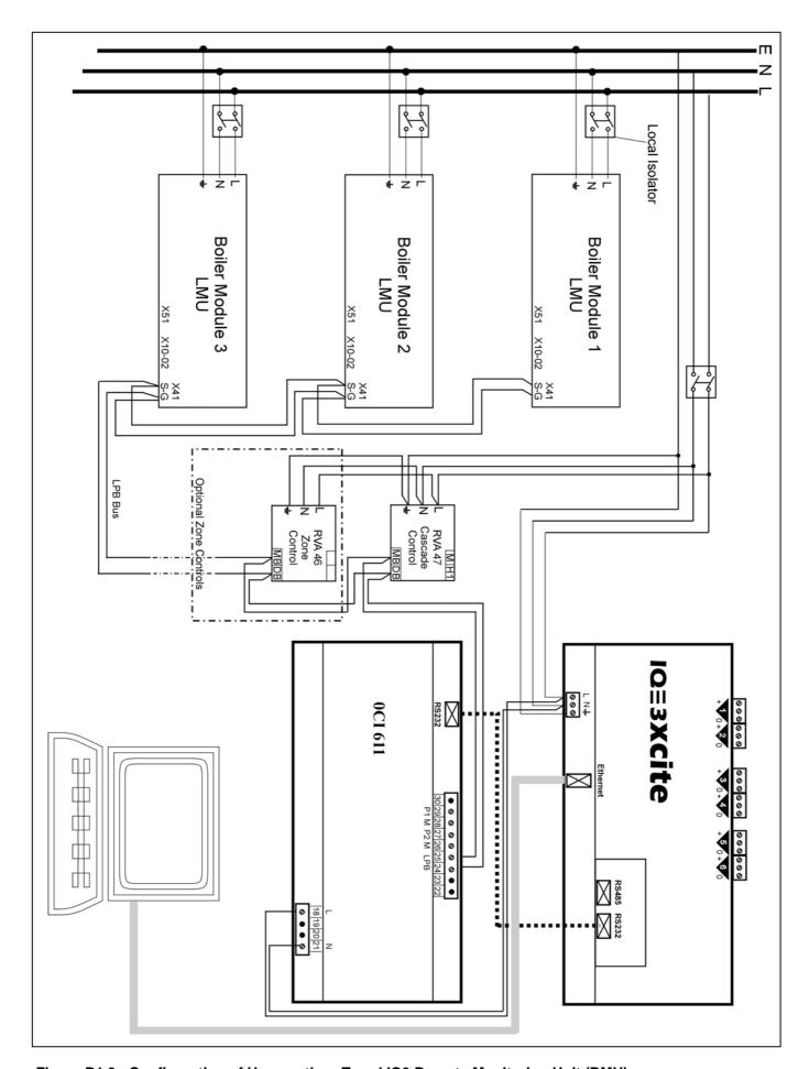
Figure B1.3 - Configuration of Hamworthy—Trend IQ3 Remote Monitoring Unit (RMU)
