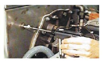
4. Insert probe horizontally into combustion chamber until depth stop is met.
