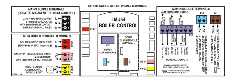
Figure 4.6 - Siemens Electrical Connections
