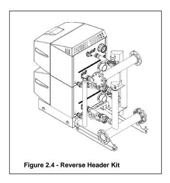
Where reverse return header sets are used these are packaged separately from the boilers. The packaging for each header set is defined in the table below. Ancillary items such as isolation valves and flexible boiler connectors are packaged in a cardboard box on the same pallet. The whole is shrink wrapped for security and basic protection.
