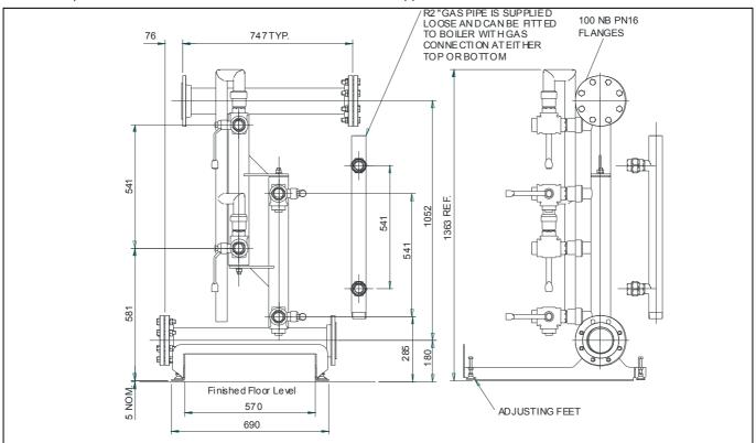
Figure 3.2.1.1 - Manifold Dimensions for ModuMax 100/200c, 110/220he, 120/240c
