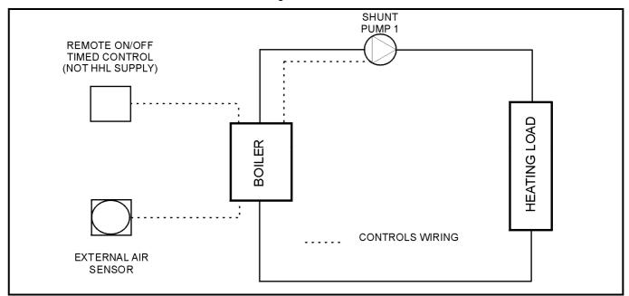
Figure E 1.3.1 - Schematic for Single Boiler System
