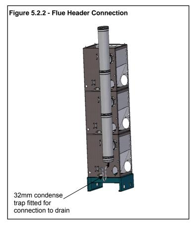
Prior to fitting the flue collector assembly, check all water and gas connections for soundness.
