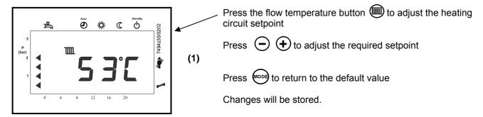
Figure 8.2.5 - Heating circuit setpoint temperature
