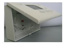
Step 2 Connect the bus cable to the screw teminals.
