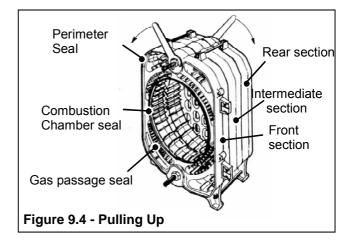
9.5.9 Select the next intermediate section and following steps 9.5.4 to 9.5.8 assemble it to the rear/
