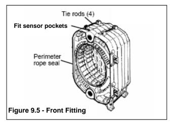
9.5.11 Prior to finally releasing and withdrawing the pulling-up bars, select the four tie rods and slide them into position, two at the top of the sections and two through the feet. Add 3 off spring washers, 1 off plain washer and 1 off nut (all M16) to each of the eight thread ends and secure but do not overtighten. Compress the spring washers by approximately 50%.
