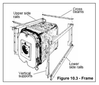
10.3.1 Assemble the four vertical supports to the corners of the boiler block using the screws, nuts and washers supplied. The supports with the deeper offset and shallower cut-out are the rear supports (See Fig. 10.3). Both the front and rear vertical supports <u>bolt to the front of the cast lugs</u> on the front and rear sections.
