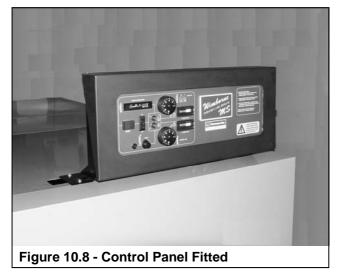
**Note:** Before fitting the control panel ensure that at least the top panel of the front casing has been removed.
