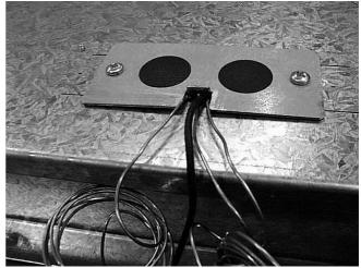
Figure 10.9 – Thermostat Capillaries exiting the Gland Plate
