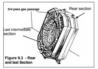
9.5.4 Select one intermediate section and identify the side with tongues instead of grooves for the gas passage seals. Apply a smooth even coating of 'Permatex' sealant to the nipple ports on this side.
