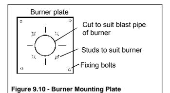
Fit the plate to the boiler door using the four longer M12 bolts and washers ensuring that the rope seal is in position and in good condition on the boiler door. Tighten the bolts sufficiently to effectively seal between the plate and the door.
