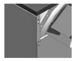
8. After mounting burner on burner mounting plate, fit plastic strikers and latches to upper and lower covers and side covers then snap covers into place. Note: Attach edging to bare edges of upper top panel.
