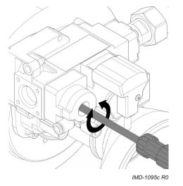
Fig. DR-FC 25 to 60 - CO<sub>2</sub> adjustment (partial load)
