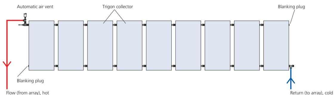
Collector array arrangements complete with hydraulic fittings kit: temperature sensor pocket and sensor, balancing valve for the collector array, automatic air vent (AAV), 3 x Tee connectors (1 capped, 1 with sensor pocket, 1 with AAV and connection nipple), 2 x blanking plugs. Each collector is supplied complete with captive unions and high temperature sealing washers. The appropriate number of flexible connectors are supplied as part of the selected collector mounting kit.
