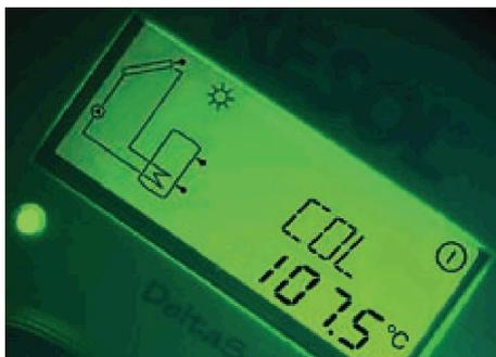
The Trigon standard and advanced solar controllers' principle function is very similar and relatively simple, i.e. it is the on/off and speed control of the solar pump in the solar transfer station under differential temperature ( $\Delta T$ ), thermostat and timer control. The generic functions common to both controllers are described here with default settings taken from the standard controller and parameter names shown in italics.
