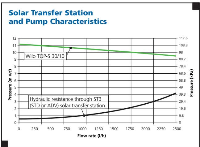
Trigon ST3 (STD or ADV) solar transfer station hydraulic resistance and Wilco TOP-S 30/10 pump flow characteristics
