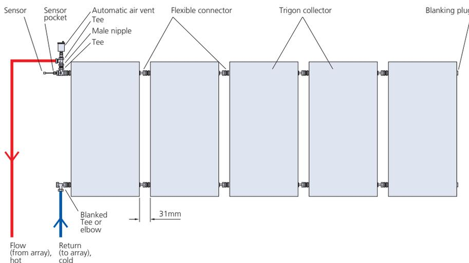
Note: The collectors have connections that extend further from the collector's body on one side than the other.
