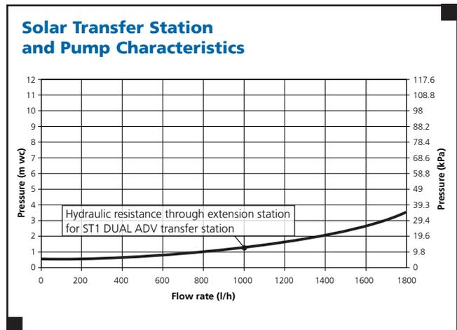
Trigon ST1 DUAL extension hydraulic resistance characteristics (For pump flow and ST1 characteristics see Wilo Star ST15/7 ECO-3 and ST1 above)
