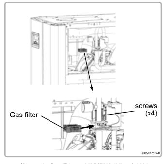
figure 46 - Gas filter on VARMAX 120 and 140
