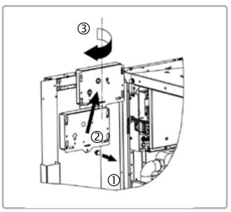
figure 7 - Unlocking the control panel
