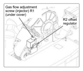
figure 45 - Gas valve models 525 and 600
