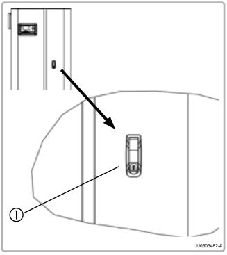
figure 6 - Opening casing doors
