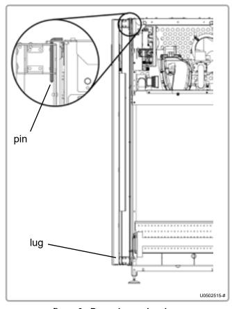
figure 9 - Removing casing doors
