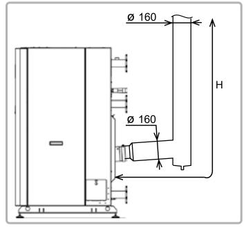
figure 21 - B23P (Ubbink) sizing recommendations
