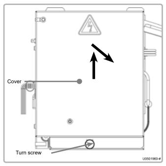
figure 30 - Opening the electrical box
