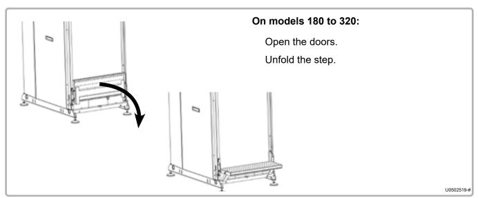
figure 14 - Installing the step on models 180-320
