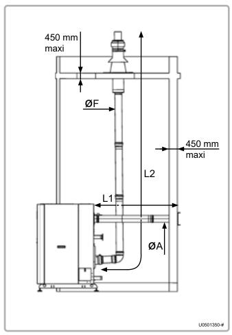
figure 25 - Type C53 connection (VARMAX models 120 to 225)
