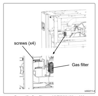
figure 47 - Gas filter on VARMAX 180 to 600
