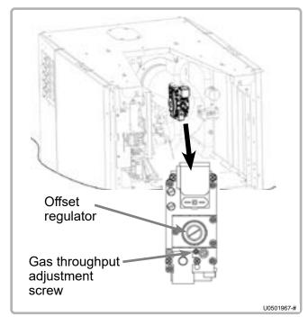
figure 43 - VARMAX gas valve models 120 and 140
