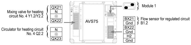
(for heating circuit shown in dots on the hydraulic diagrams)
