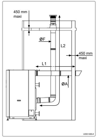
figure 26 - Type C53 connection (VARMAX models 275 to 600)
