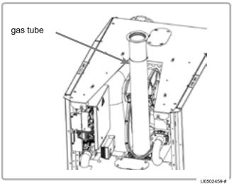
figure 56 - Cleaning the gas tube
