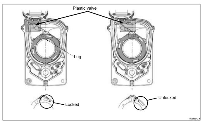
figure 55 - Positions of the fastening clamps
