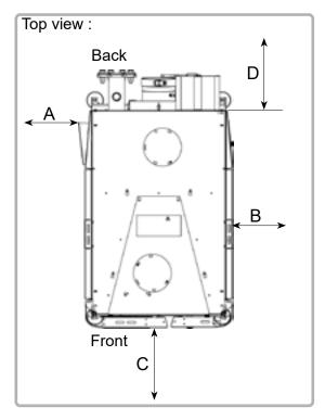
figure 4 - Peripheral clearance
