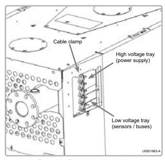
figure 31 - Electrical cable bushing
