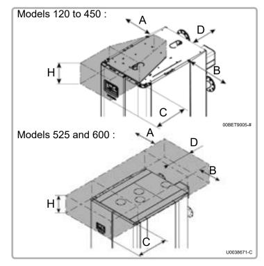
figure 5 - Specific clearances required for burner maintenance operations
