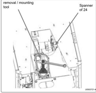
figure 54 - Release the burner tube
