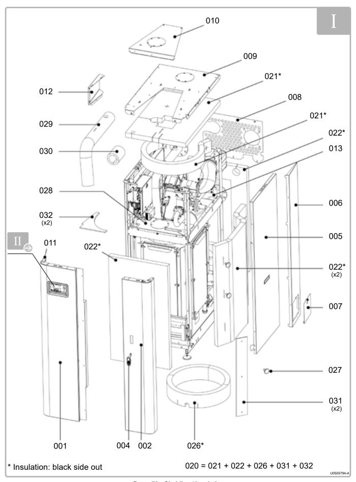
figure 72 - Cladding / Insulation
