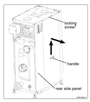
figure 10 - Removing side panels
