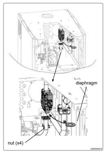
figure 16 - Diaphragm (120 and 140 models)
