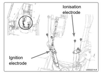
figure 37 - Position of electrodes
