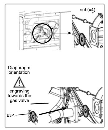
figure 17 - Diaphragm (275 and 320 models)
