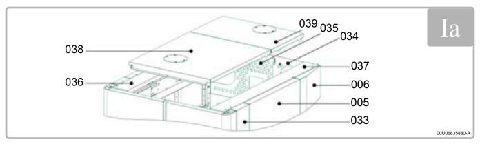
figure 73 - Specific casing 525 and 600 kW
