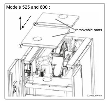
figure 12 - Disassembly of upper panels
