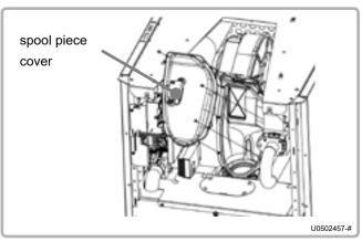
figure 53 - Removal of spool piece cover
