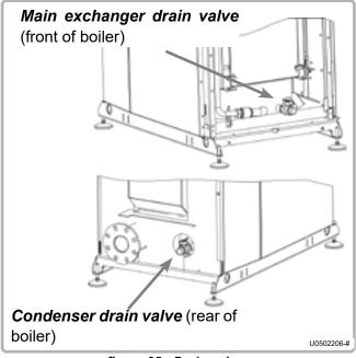
figure 35 - Drain valves
