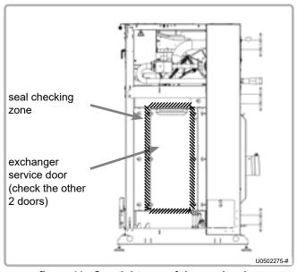
figure 41 - Gas-tightness of the service door
