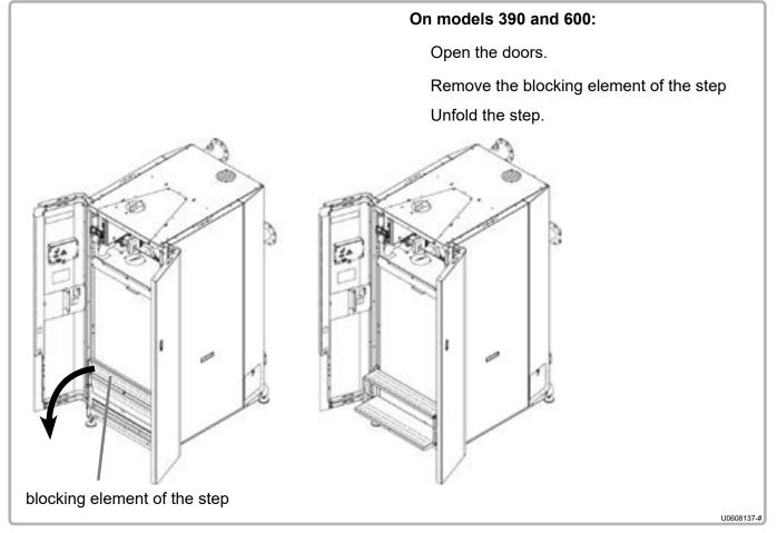
figure 15 - Installing the step on models 390 and 600
