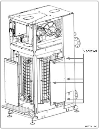
figure 48 - Removal of exchanger doors
