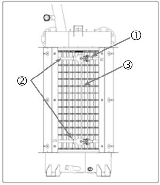
figure 49 - Removal of baffles
