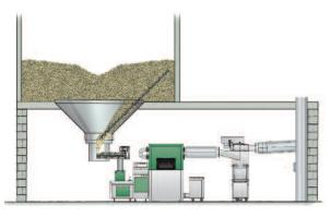
Storage room is above plant room. Discharge via pendulum screw from silo.
