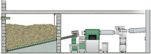
Transportation of pellets with inclined discharge screw.
