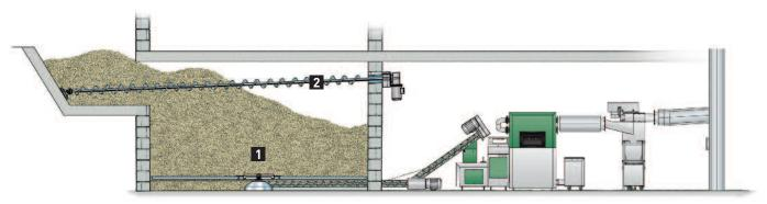
Storage room discharge via horizontal spring agitator (1) with rising screw allows optimum usage of the fuel storage room. The filling screw (2) distributes chip evenly during delivery
