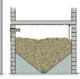
For systems without a spring agitator the hopper base should slope at a minimum angle of 45 degrees towards the central auger
