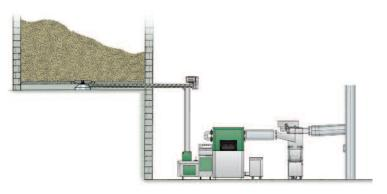
Storage room and plant room are on different levels. Horizontal discharge with spring agitator and falling chute.
