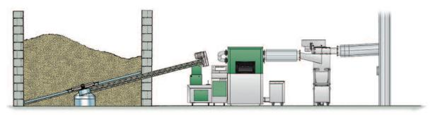
Storage room and heating room are on same level. Transversal discharge with spring agitator.
