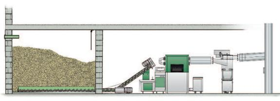
Horizontal pellet discharge from the storage room, with rising auger to optimise storage space.
