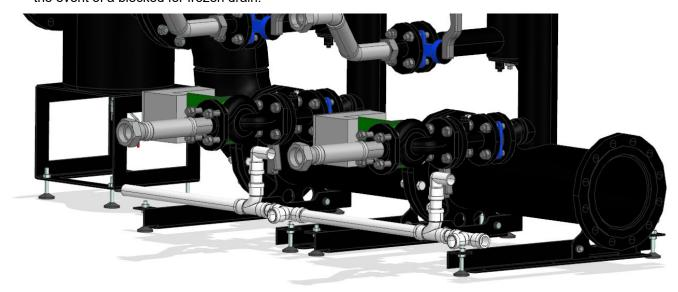
Figure 4.6 Condensate Pipe Position
