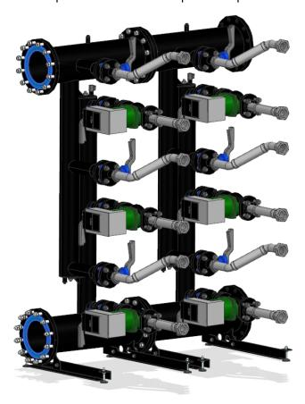
Figure 4.1 Additional Flow and Return Manifold
