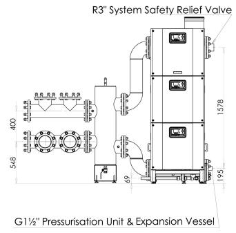
Figure 1.2.2 - DN150 2H / 3H Primary circuit and Gas manifold pipe kit
