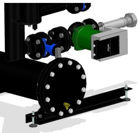
Figure 4.2 Blanking Flange Position
