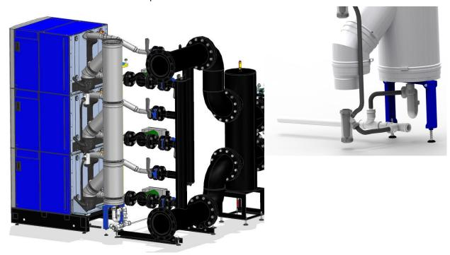
Figure 4.11 Flue Manifold and Drain Pipe Work
