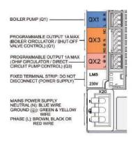
The contactor/relay will need a separate 230v supply, rated at the correct pump current rating to feed the pump terminals at the pump L, N & E (PE). The signal from QX1 will operate the contactor/relay to operate the pump.
