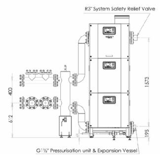
Figure 1.2.1 - DN100 2H / 3H Primary circuit and Gas manifold pipe kit
