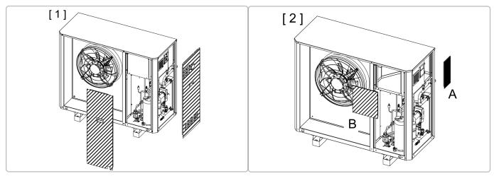
Figure 2 - Dismantling procedure
