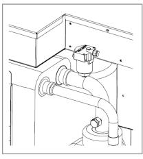
Figure 12 - Automatic air trap
