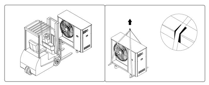
Figure 4 - Lifting with a fork lift truck
