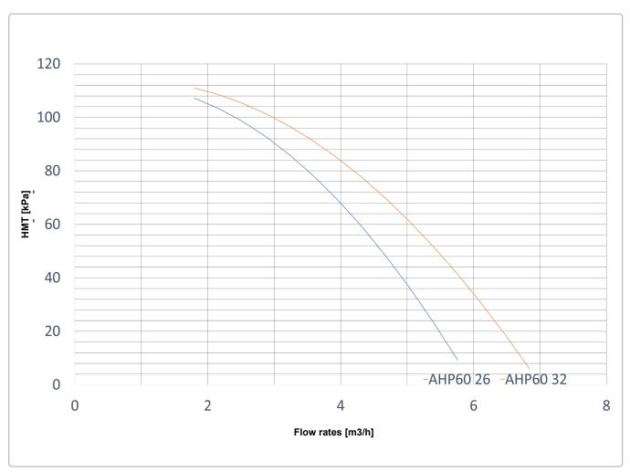
Figure 10 - Hydraulic pressures and flow rates available
