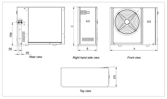
Figure 1 - Frame sizes (in mm) for both 26kW and 32kW
