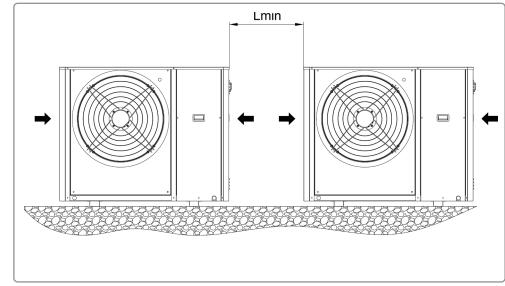
• If units are positioned side by side, the minimum distance Lmin to be respected between them is 700mm.
