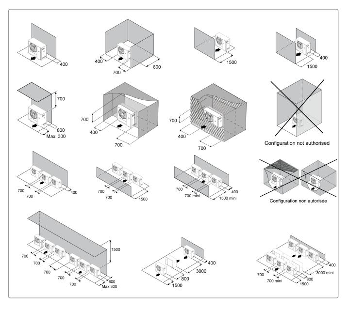
Figure 8 - Minimum clearances and types of installation
