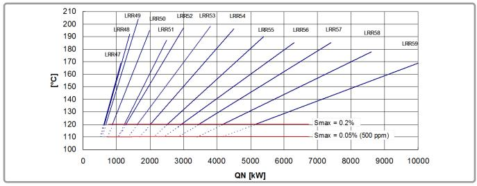
figure 7 - Flue gas temperature diagram LRR, fuel oil with clean boiler
