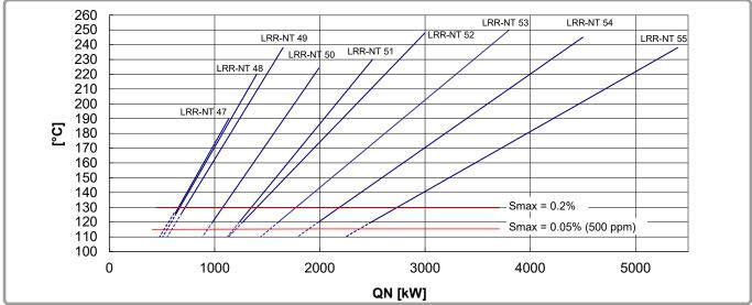
figure 9 - Flue gas temperature diagram LRR-NT, fuel oil with clean boiler
