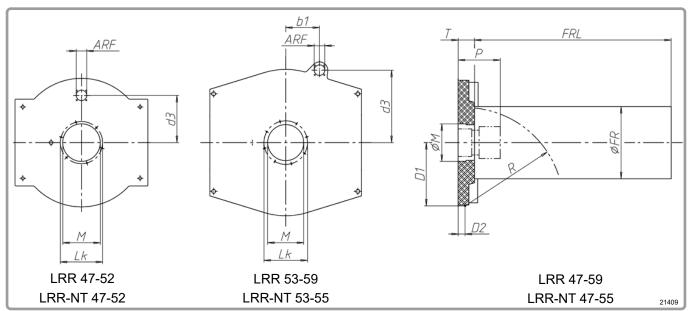
figure 16 - Burner mating dimensions for LRR / LRR-NT
