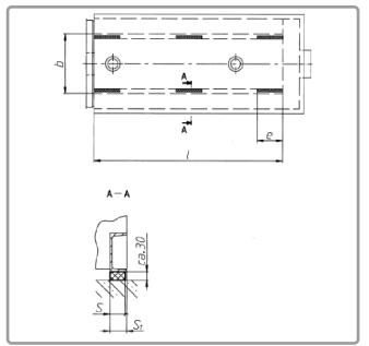
figure 13 - With vibration dampers
