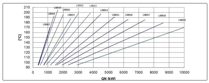
figure 8 - Flue gas temperature diagram LRR, natural gas with clean boiler
