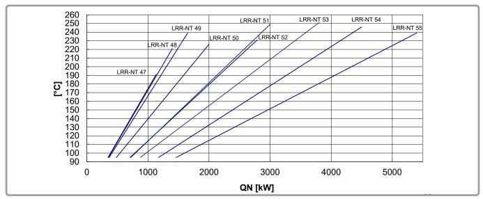
figure 10 - Flue gas temperature diagram LRR-NT, natural gas with clean boiler
