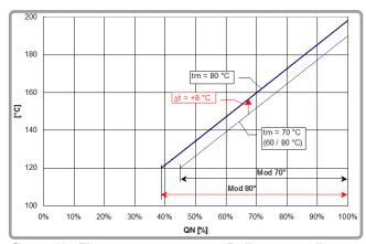
figure 11 - Flue gas temperature – Boiler power diagram (example for two average boiler water temperatures)
