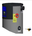
The Temperature and Pressure Relief Valve must be fitted and should not be disconnected other than for replacement. The Temperature and Pressure Relief valve will open if the pressure or temperature within the tank exceeds the valve limit. The DR-SG water heaters are provided as standard with a 7 bar / 90°C T&P relief valve. If the valve is activated, it will remain open until the water has dropped below the unsafe temperature and pressure limit.
