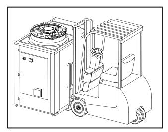
Figure 5 - Lifting with a fork lift truck
