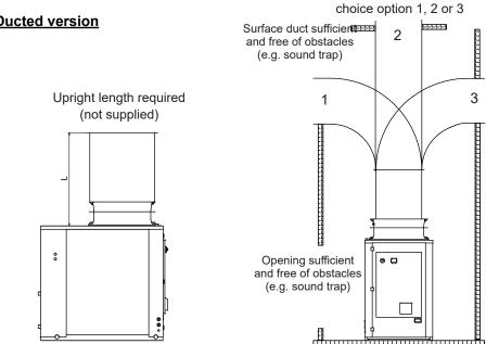
The figure shows an example of a possible ducted installation. Before making any change to the direction of the duct, the minimum length to be observed is indicated (L = 1 m). The following is a quantitative indication of the additional static height that can be obtained with the ducted version compared to the standard version, with the same flow rate and the same absorbed power. Pressure drops that are any greater will not guarantee the declared performance.
