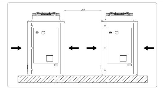
• If units are positioned side by side, the minimum distance Lmin to be respected between them must be a minimum of 2.20m. The figure below shows the different cases.
