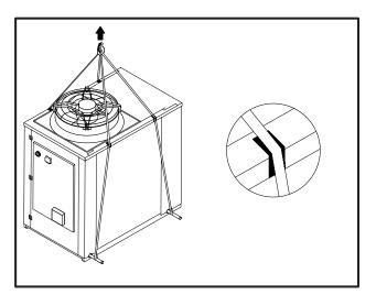
Figure 6 - Lifting with ropes/chains and sling bars
