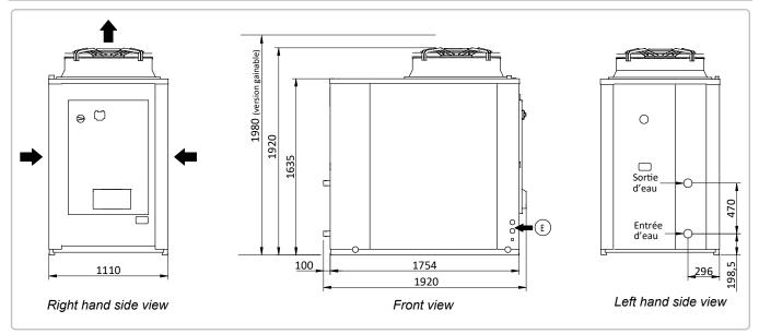
Figure 1 - Dimensions of the models AHP60 50 - 70 kW
