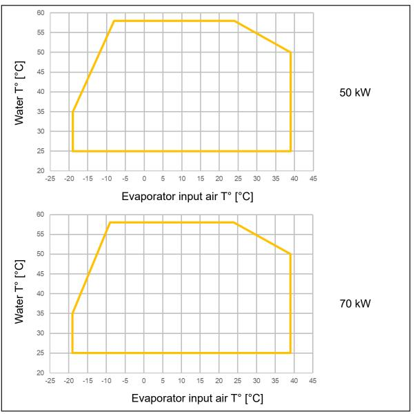
Range of water supply temperatures depending on the ambient temperature:
