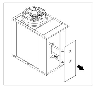
In case of maintenance and/or checking of the hydraulic component and the refrigeration circuit, it is necessary to access the inside of the unit through the rear panel, which is close to the hydraulic connections.
