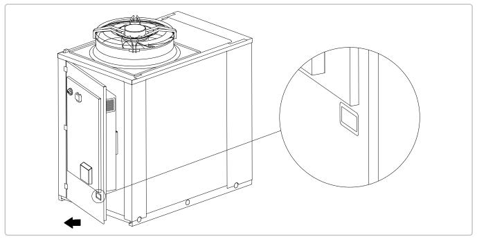
Figure 2 - Access to the refrigeration component
