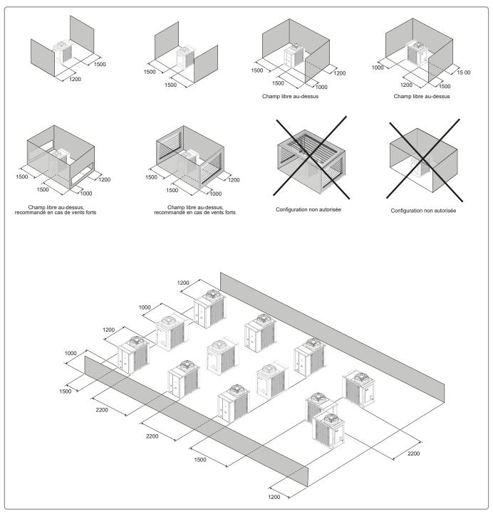
Figure 8 - Minimum clearances and types of installation
