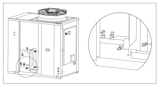
Figure 12 - Safety valve location
