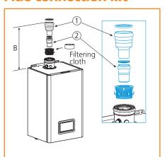
**B** indicates the height of the of the chimney adapter when fully inserted relative to the upper panel of the boiler.
