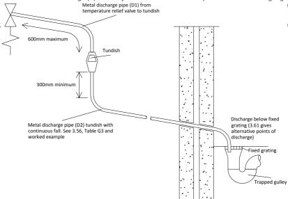
Figure G3: Typical discharge pipe arrangement
