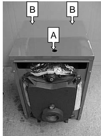
Push the top cover onto the location studs in the top edge of the side cover. Making sure the cable entry hole (A) is at the front of the boiler. Secure the top cover to the rear cover using the 4x10 self tapping screws (B).
