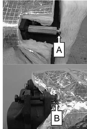
View showing the front (B) and rear (A) connection points for the side covers.
