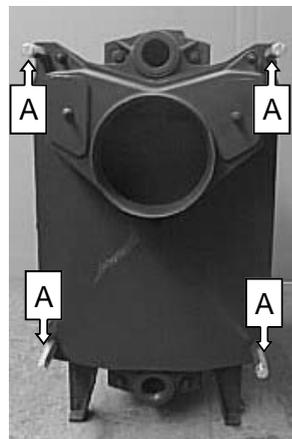
Screw the four 80mm spacers on to the ends of the tie rods and partly screw in the four M10x15 bolts into the ends of the spacers.
