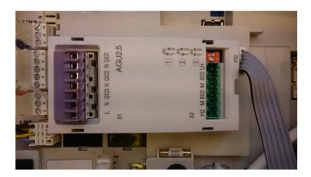
6 Fit the other end of the grey ribbon cable into X50 on the Navistem controller as shown below.
