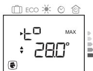
Set the maximum temperature of your choice by pressing on or . After 5 seconds on one activity, the temperature is automatically validated.
