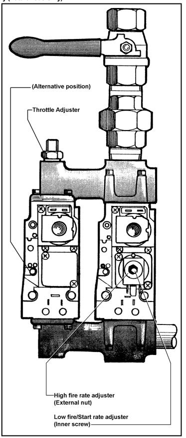
For Natural Gas the gas pressure governor control system is configured for a nominal gas inlet pressure of 20mbar with a maximum inlet pressure of 25mbar. The Warmwell 120 and 140 boiler is fitted with a unique flow share gas valve arrangement. Refer to Figure 11.7b (p30) to establish method of adjustment of the by-pass throttle arrangement. NOTE! The by-pass valve throttle MUST only be used as a coarse adjuster, the main control MUST always be accomplished by the high/low control valve.
