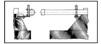
Tighten screws ensuring 'U' clamp threads do not damage insulation. It may be necessary to remove the bottom thread of the 'U' clamp with the bracket in lower position as it may foul the draught hood. Ensure no undue stress is placed on the gas pipe/manifold and ensure pipe is vertical/horizontal before clamping in position.
