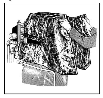
Refer to Figure 10.2.2c - Close flaps around bottom of secondary heat exchanger. Ensure unit is completely covered. The insulation jacket should not cover the stainless steel collector hood.
