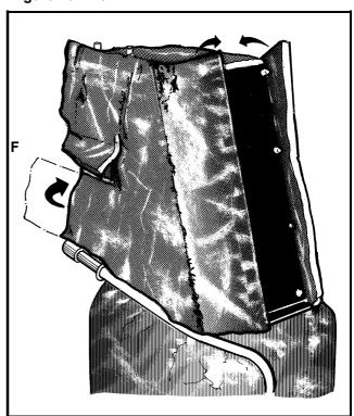
Seal all joints with tape provided. Loosely close the front flaps covering the inspection door. Place two pieces of tape on front split to allow access to the inspection door.
