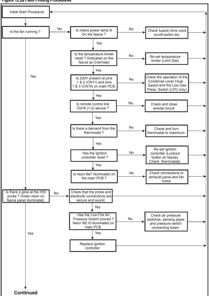
Figure 12.2b Fault Finding Procedures (Cont.)
