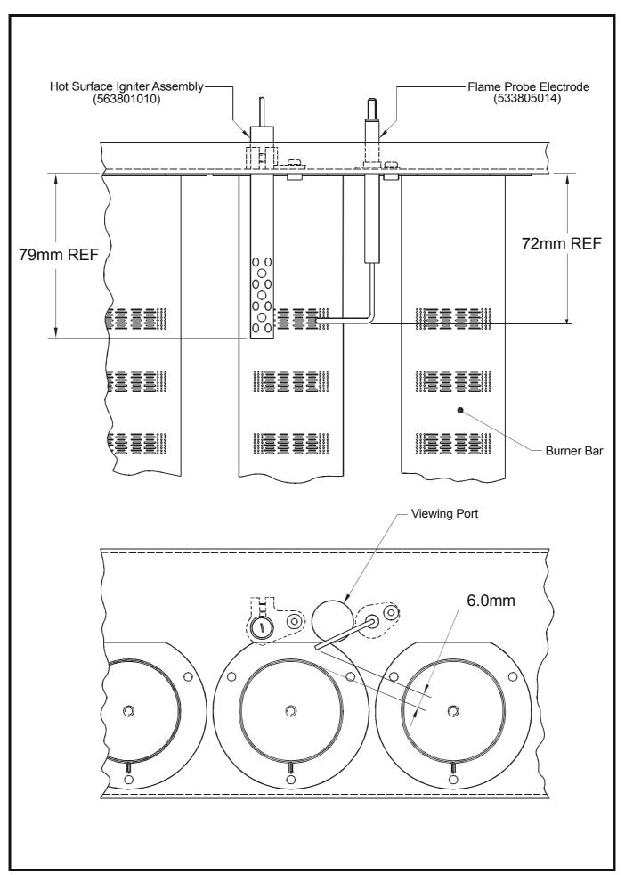
that of the control thermostat with some minor differences. These are as below: -
