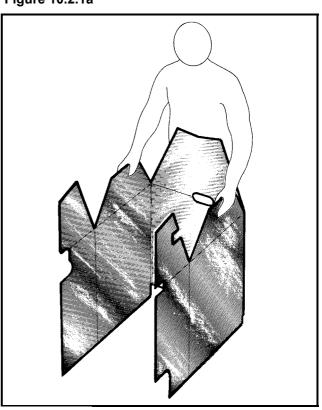
Reference to Figure 10.2.1b - Insulation should be folded around boiler such that its rear edges meet in the centre. Ensure flow and return connections are clear and unobstructed.
