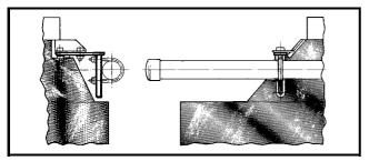
Figure 10.3c shows the pipe clamp fitted to Warmwell 60kW boilers.
