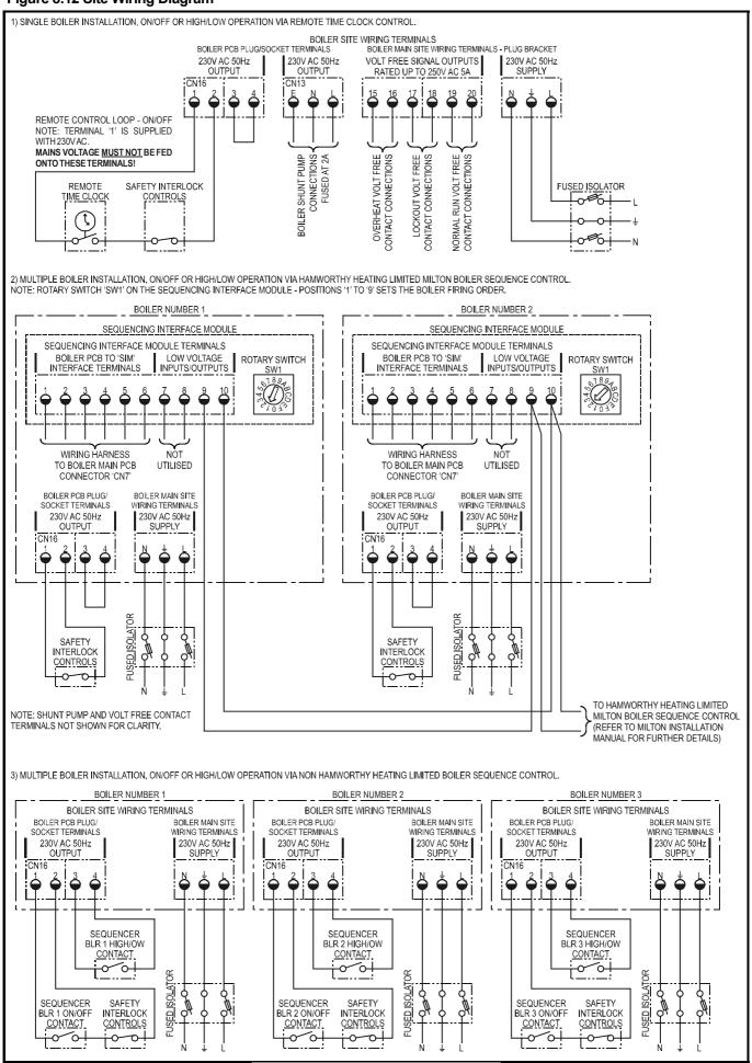
Figure 9.1 Wiring Schematic
