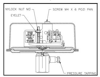
With the cover removed, turn the M3 nut clockwise to increase the set point and vice-versa. Seal the adjuster after setting.
