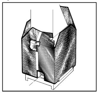
Apply foil tape down join. Leave 'petals' in upright position at the sides for installation of secondary heat exchanger insulation. Mould the rear 'petal' into the shape of the boiler and fold the front 'petal' such that the access door is not covered. Use foil tape to secure joins and folds whilst ensuring gas pipe bracket and thermostat pocket are clear and unobstructed.
