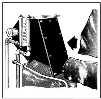
Refer to Figure 10.2.2b - Fit jacket over the transition duct and secondary heat exchanger. Ensure the two air vents protrude through the jacket. Feed jacket between the two M6 studs, which will eventually hold the casing support bar.
