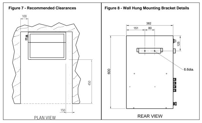
A mounting bracket is supplied inside the wall mounted unit taped to the front of the tank. It is intended that this bracket should be fixed to the wall and the unit hung from it.
