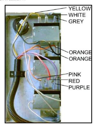
Figure 26 Switch Wiring
