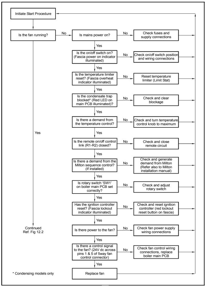
Figure 12.2. Fault Finding Procedures.
