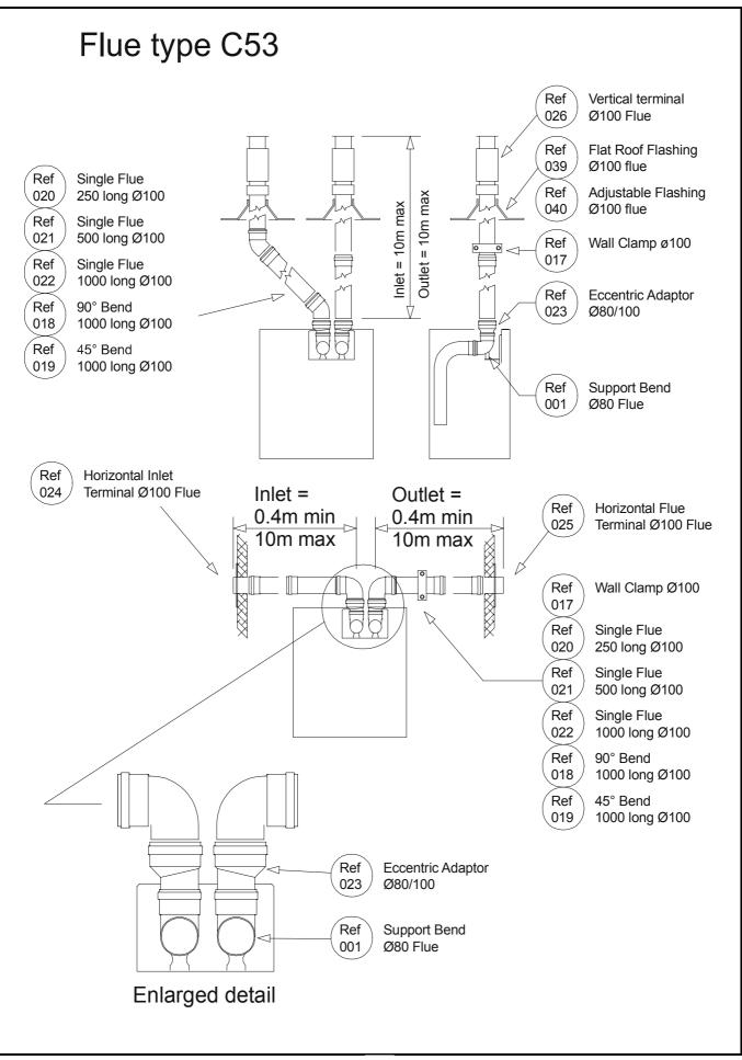
Figure 6.1.4. - Intake from Ventilated Plant Room and Discharge via Horizontal/Vertical Flue
