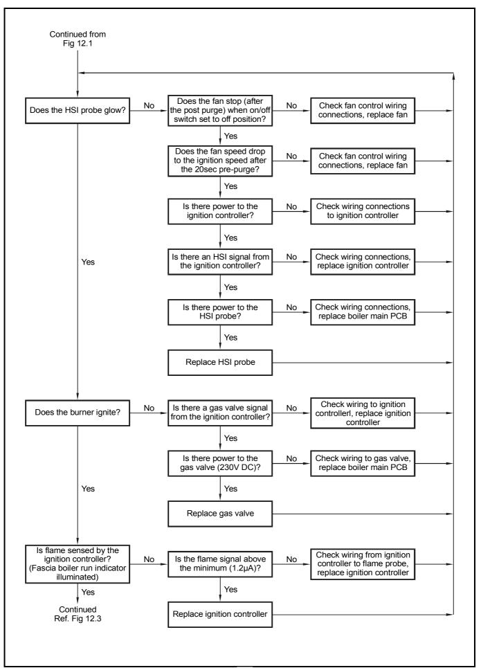
Figure 12.3. Fault Finding Procedures.
