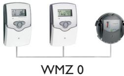
\* The maximum number of cascaded WMZ modules is 16. Whether this number can be reached depends on the construction.
