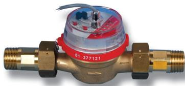
A flowmeter V40 is used in order to determine the volumetric flow rate in the solar circuit. The installation is to be carried out taking the flow direction into consideration (consider direction indication on the flowmeter). In order to tranquilise the flow ratio, an inlet and an outlet distance of 30 cm in front of and behind the flowmeter have to be taken into account.
