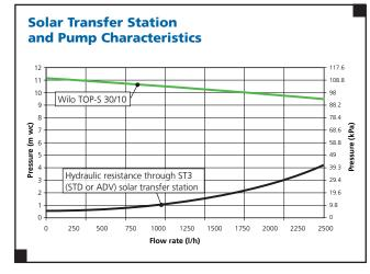
Trigon ST3 (STD or ADV) solar transfer station hydraulic resistance and Wilo TOP-S 30/10 pump flow characteristics
