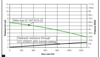
Trigon ST1 (STD or ADV) solar transfer station hydraulic resistance and Wilo Star ST15/7 ECO-3 pump flow characteristics
