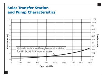
Trigon ST1 DUAL extension hydraulic resistance characteristics (For pump flow and ST1 characteristics see Wilo Star ST15/7 ECO-3 and ST1 above)
