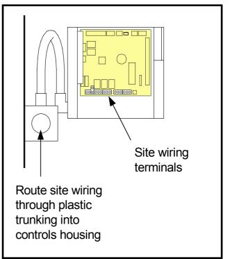
A 0-10V analogue control signal from the external sequence control system is required, ground and signal connections. The interface module is configured to give a linear response to the 0-10V signal between 2.0V (20% rate) and 10.0V (100% rate). Below the 2.0V the boiler will operate at 20% rate until the input signal falls below 0.3V at which point the boiler is shut down. There is  $\pm 0.1V$  switching hysteresis.
