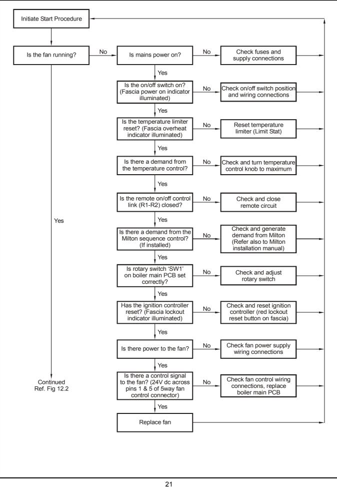
Figure 12.2 Fault Finding Procedures.
