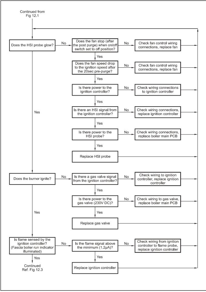
Figure 12.3. Fault Finding Procedures.
