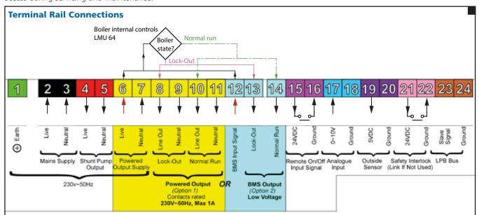
The Purewell VariHeat provides options for powering the Lock-Out/Normal Run indication function by a choice of either 230 VAC mains or by a low voltage (typically 12V or 24V DC) supplied from a BMS. A choice of two sets of terminals, Option1 (yellow terminals 6 to 11) for 230 VAC mains signalling and Option 2 (pale blue terminals 12 to 14) for Low Voltage signalling have been provided for the Lock-Out/Normal run indication function. Note that only one option may be selected.
