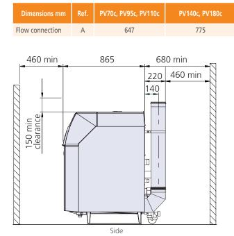
Note: Do not run trunking or pipework across the top of the boiler. Access is required top and front for servicing. All dimensions in mm unless otherwise stated.
