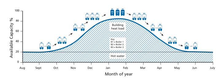
The overall efficiency of a multiple boiler plant depends on how close its total output can be controlled to match the load profile of the building. Therefore, it is a really important aspect of product selection.
