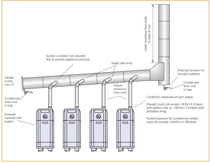
Multiple Purewell Variheat mk2 boilers sharing a common flue header and B23 type flue
