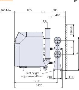
For 4 boilers use 2 x 2-boiler pipe kit, width 2336\*
