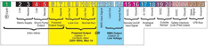
The following electrical connections are provided on each module on a rail at the base of the front of the boiler:
