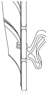
A line drawing showing the peg fully inserted into the slot of the strip. The hand is no longer present.                                        |
